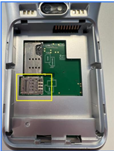
4. Insert the SIM by sliding it towards the left into the SIM card holder. Make sure the SIM is inserted in the correct way (as the diagram below shows).
