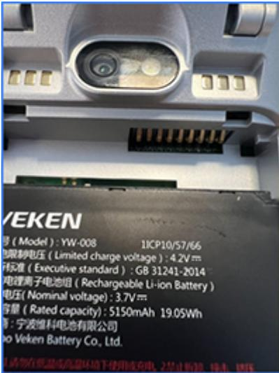
6. Once the battery is re-inserted, place the back of the terminal back onto the Verofy® Move. To secure in place, move the lock mechanism to the left to lock the back panel in place.
