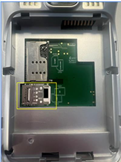
4. To remove it, carefully slide the SIM card to the right to release it from the SIM holder.
